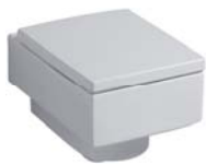
Wash-down WC, 6 l, wall-hung, 350 x 530 mm, model-no. 203200. WC seat with soft closing mechanism, Model-no. 571280. Can be combined with Keramag Design sanitary modul Universal.
