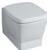
Wash-out WC, 6 l, wall-hung, 360 x 540 mm, raised seat height (+ 30 mm, when installed with standard mounting dimensions), model-no. 203670. WC seat with soft closing mechanism, model-no. 572620. Can be combined with Keramag Design sanitary modul Universal.
