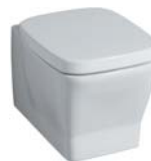
Wash-down WC, 6 l, wall-hung, 360 x 540 mm, raised seat height (+ 30 mm, when installed with standard mounting dimensions), model-no. 203650. WC seat with soft closing mechanism, model-no. 572620. Can be combined with Keramag Design sanitary modul Universal.
