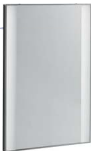
Illuminated mirror, frame polished stainless steel, 2 T5 lamps FH 21 W, RGB LEDs, 220-240 V~, 50-60 Hz, IP44, protection class 2, anti-condensation, light switch, remote control, 600 x 900 x 55 mm, model-no. 816560.
