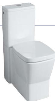
Wash-down WC combination, 6 l, floor-standing, 360 x 850 x 670 mm, model-no. 203600. Ceramic cistern with dual flush 3 l/6 l, water supply from side/rear, model-no. 227630. WC seat, model-no. 572620.
