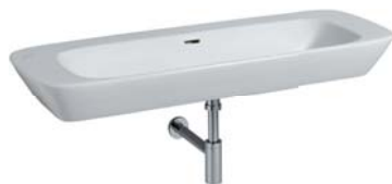
Washbasin without tap holes, one tap hole punched out in centre, 1200 x 470 mm, model-no. 121625. Can be combined with washbasin plates, siphon cutout centre, 1200 · 1400 mm and washbasin vanity units 1200 · 1400 mm.
